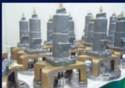
Ballast Control Valve - 2
